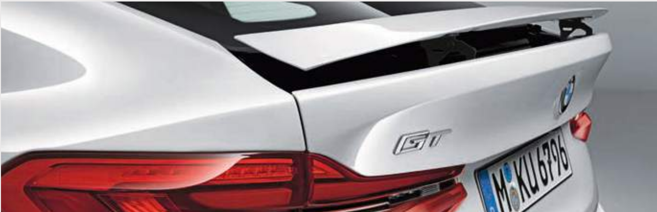
The Active Rear Spoiler automatically extends at a speed of over 110 km/h and retracts once the speed returns to 70 km/h in order to improve stability.
