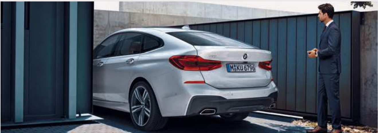
The Remote Control Parking function allows the driver to conveniently get out of the vehicle before parking it via remote control by moving it forward into, or reversing out of a tight parking space or garage. The Remote Control Parking function is activated by the driver once outside the car, with the BMW display key.
