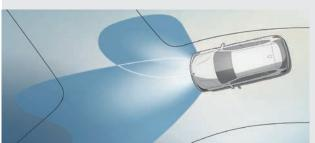
**LED Headlights** with low-beam and high-beamusing BI-LED technology as well as direction indicators in full LED technology. The equipment also features cornering lights and daytime running lights that help improve driving safety by optimally illuminating the road ahead..
