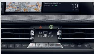
The **Automatic Air Conditioning with 2-Zone Control** and automatic target temperature control features separate controls for you and your front passenger. It also includes Automatic Air Recirculation (AAR), a micro-activated carbon particulate filter, a fogging and solar sensor, as well as rear air vents.
