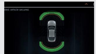
Parking Assistant makes parking the vehicle easier. The Rear-View camera provides a clearer view behind the vehicle. Active Park Distance Control offers increased protection against damage caused by parking. Parking Assistant parks the vehicle automatically, parallel or perpendicular to the street, and leaves parallel parking spaces. The Reversing Assistant supports you when reversing, e.g. in narrow lanes.
