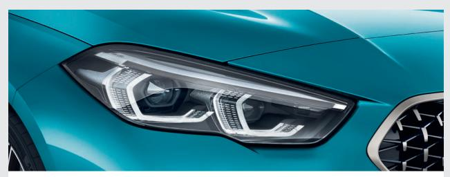
**LED Headlights** with low beam and high-beam using BI-LED technology as well as direction indicators in full LED technology. The equipment also features cornering lights and daytime running lights that help improve driving safety by optimally illuminating the road ahead.
