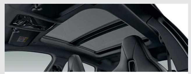
When open, the **Panorama Glass Roof** provides a great deal of fresh air. Closed, it creates a bright, light-flooded atmosphere in the interior. It opens and closes completely automatically at the push of a button or with the vehicle key and is equipped with slide and lift functions, a roller sunblind and wind deflector.
