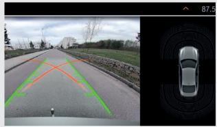
The **Reversing Assistant** records up to 50 m of the road you have driven forwards so that it can reverse the vehicle automatically in the same direction if you wish. The distance of the remaining route is shown in the image of the Rear View camera.
