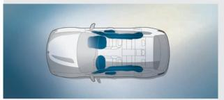
**Airbags for driver and front passenger** are an integral part of the optimally coordinated safety components in a BMW. A total of six airbags offer targeted protection: driver and front passenger airbags, head airbags for the whole side window area, and side airbags in the front seat backrests.
