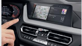
With **BMW Gesture Control**, selected functions can be operated by means of defined hand movements. Simple gestures such as 'swiping' or 'pointing' are identified in the recognition area above the centre console and trigger functions such as accepting or rejecting an incoming telephone call, proceeding or cancelling navigation as well as starting and ending voice recordings.
