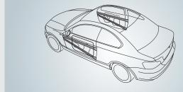
**Side-Impact Protection** ensures greater safety. Thanks to the directions of the beams and node joints and selective use of high-strength materials, the functionally designed passenger cell structure provides maximum passive safety in the event of a front, side or rear impact.
