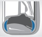
**The Runflat Indicator (TDI)** warns the driver with a light in the Control Display when there is a slight drop in tyre pressure. When there is a large pressure drop, there is an additional acoustic warning.
