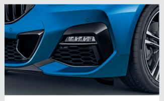
**LED Fog Lights** increase short-range visibility in fog or precipitation, improving night-time driving safety.
