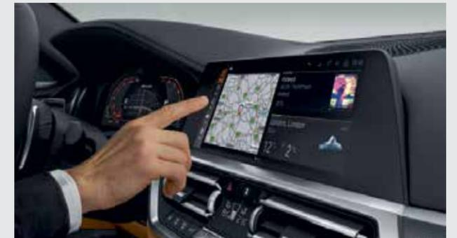
With **BMW Gesture Control**, selected functions can be operated by means of defined hand movements. Simple gestures such as 'swiping' or 'pointing' are identified in the recognition area above the centre console and trigger functions such as accepting or rejecting an incoming telephone call, proceeding or cancelling navigation as well as starting and ending voice recordings.
