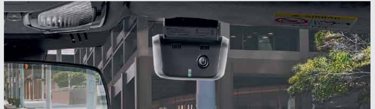
**Advanced Car Eye 2.0.** A highly sensitive full-HD camera that captures events in front and behind the car, even when it is parked. In the event of disturbances and extraordinary movement outside the vehicle, the camera automatically records the situation in order to document possible accidents or (attempted) break-ins.
