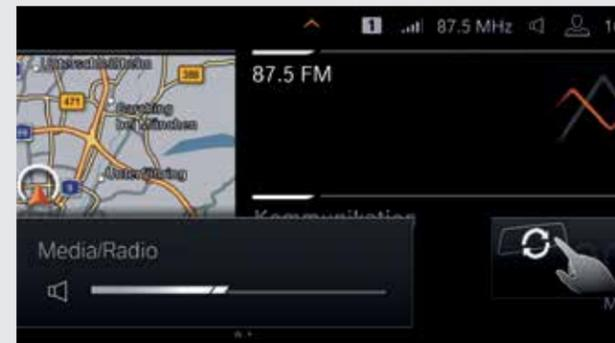
With **BMW Gesture Control**, certain functions can be operated by means of defined hand movements. For certain operations the system will, for example, recognise gestures such as 'swiping' or 'pointing' for accepting or rejecting an incoming call, or circular motions of the index finger to adjust volume.
