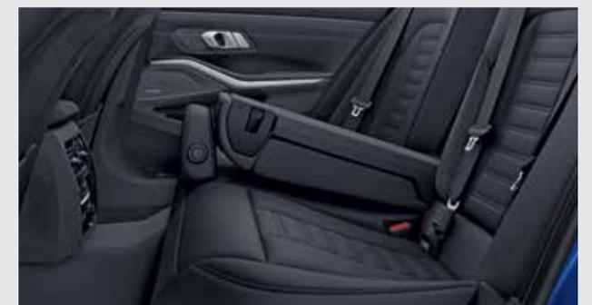
The through-loading system includes rear seat backrests that can be divided in a 40:20:40 ratio for the greatest possible flexibility. For example, two passengers can be seated comfortably in the rear, while long objects such as golf bags can be transported at the same time. The two cupholders in the centre armrest are very practical.
