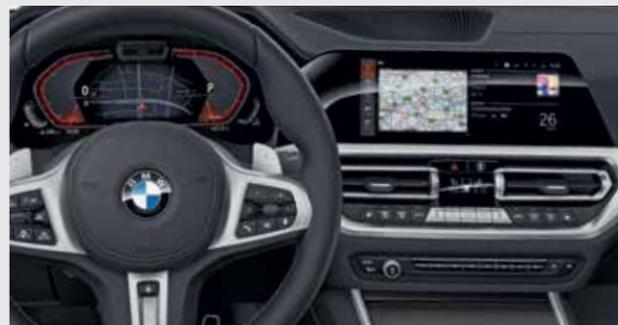
The BMW Live Cockpit Professional with navigation function includes a high-quality display network consisting of a high-resolution 10.25" (26 cm) Control Display that can be operated by touch and a fully digital 12.3" (31.24 cm) instrument display. The BMW Operating System 7.0 can also be operated via the iDrive Controller.
